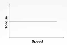
The load torque demand does not change regardless of the running speed. Most friction loads such as conveyors, cranes, saws etc. are good examples of this type.
